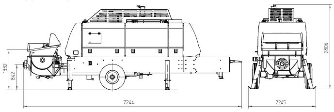
Note: Standard version BSA 2110 HP D4. Dimensions and weights depend on equipment. Subject to technical modifications and errors.
