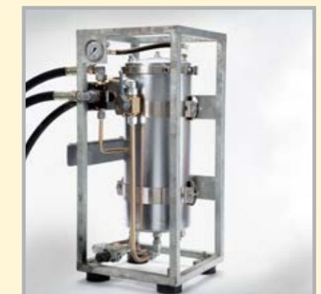
The mobile partial flow filter extends life and reduces oil changes
