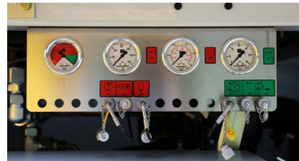
Mini-measuring strip: All hydraulic measuring points at a central location (BSA latest generation)
