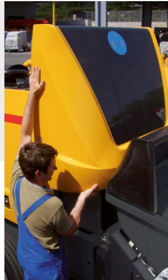
GRP hood: robust, weather-resistant and easy to remove
