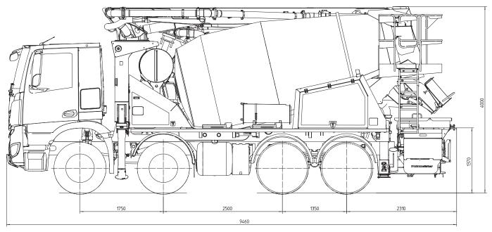
Note: Standard version. Subject to technical modifications and errors. Dimensions in mm, for example MB-Arocs, dimensions depending on the vehicle. Pictures contain optional equipments.
