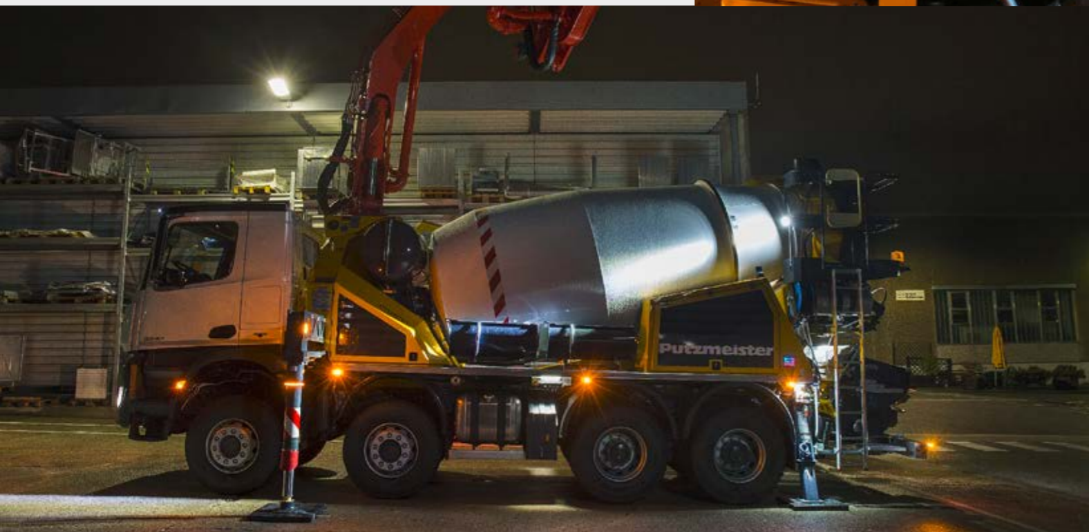
The new lighting concept for illuminating the operating points and the support ranges offers not only comfort, but also more safety around the machine
