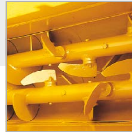
Twin-screw auger feeding device with mixing paddles in the supply chute
