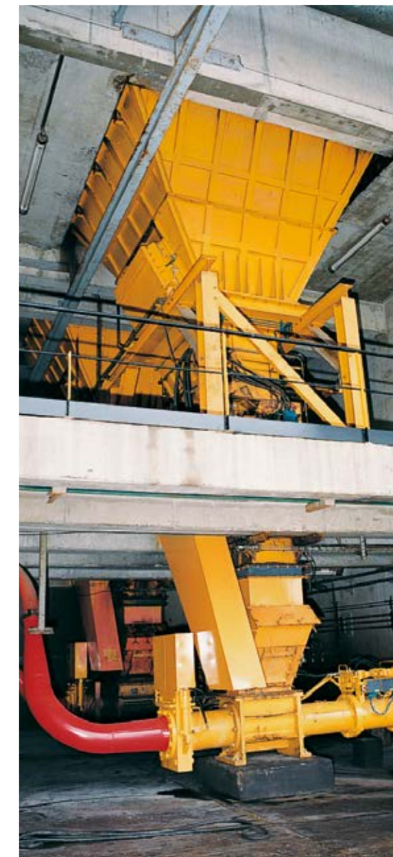
EKO 14100 feeding the rotary kiln with shredded barrel waste in a hazardous waste treatment plant
