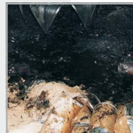
Coarse hazardous waste from the reception bunkers is fed via claw arm to the EKO piston pump
