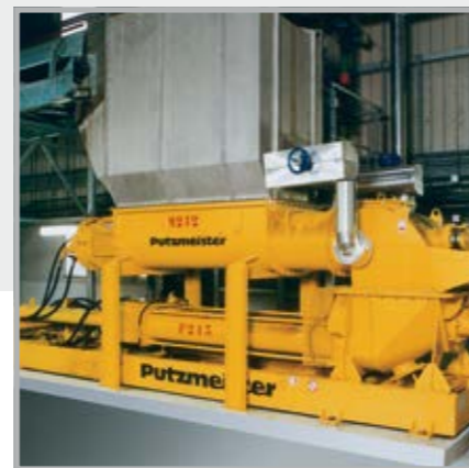
Biowaste recycling plant in Varenne-Jarcy, France: KOS 2180 pumping biomass into a fermentation plant
