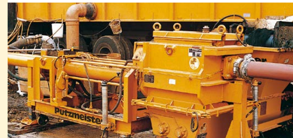
Mobile dewatering and pumping station
