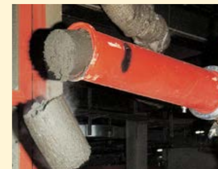
Sewage sludge from filter press and centrifuges
