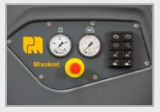
User-friendly robust keypad clearly arranged and easy to use - thanks to the "follow the blue light" principle
