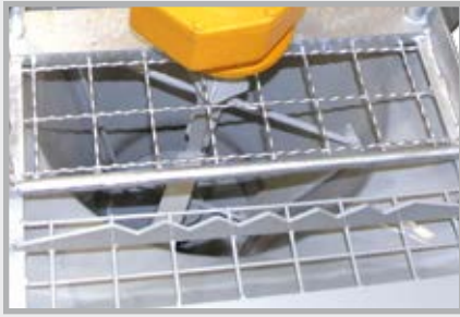
Mixing, pumping and spraying from a single material hopper
