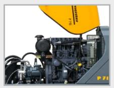
Two drive versions: Reliable oil-cooled 3-cylinder Deutz diesel engine complies with exhaust emission regulation (Stage 3A) or low-noise, environmentally friendly electric motor (30 kW)
