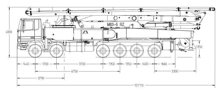
Note: Serial version. Dimensions and weights depend on truck, pump model and equipment.
