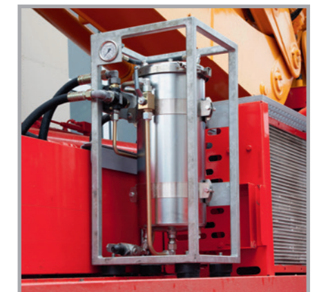
The mobile bypass filter extends service life and means oil changes are less frequent.
